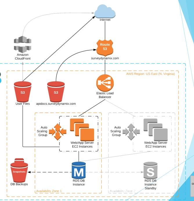
Greyed out components indicate redundancy and scalability options
